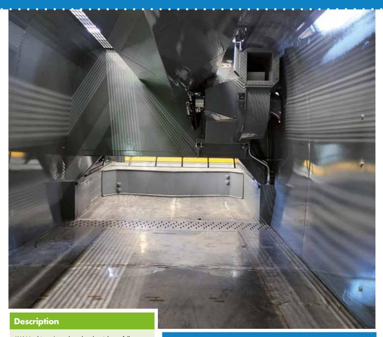
AW Machinery's wash and suck unit has a full press mechanism. Waste is compressed as many as four to five times. The design of this press block is also one of a kind. It is a double parabolic press block that ensures even distribution of the pressing force as well as minimal contamination behind the press block. It is a powerful and above all reliable mechanism.
