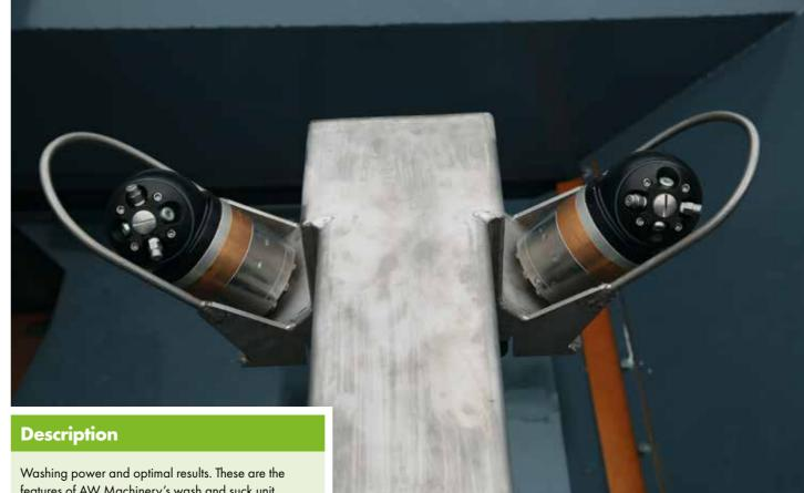
Washing power and optimal results. These are the features of AW Machinery's wash and suck unit. The patented washing arm together with the double washing heads guarantees that the water jet under high pressure cleans all corners of the valves. Manual stabbing of residual waste is now a thing of the past!
